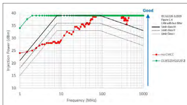
Figure 8: Results from DPI immunity test configuration using signal generator and power amplifier to inject RF noise (Source: Murata)
