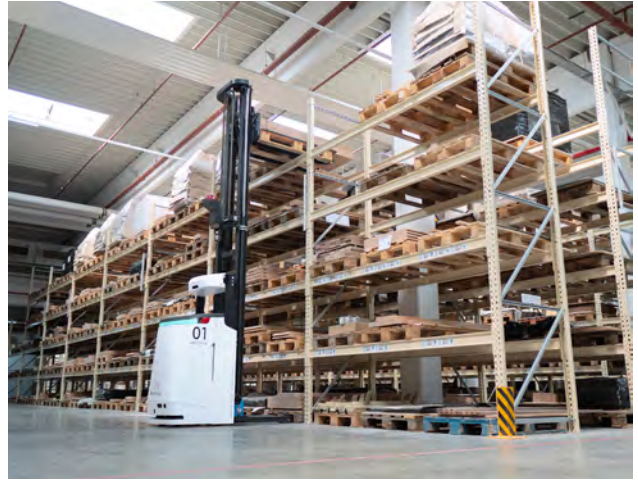
Figure 4: Transfer heights of up to 4 m are no problem with the duplex lift mast (Source: EK Robotics)
