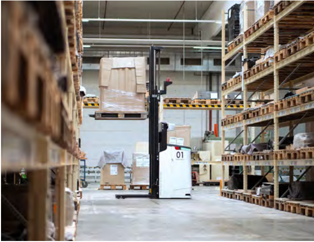
Figure 2: The vehicles serve over 900 storage locations in the shelving warehouse and move loads of up to 1000 kg (Source: EK Robotics)
