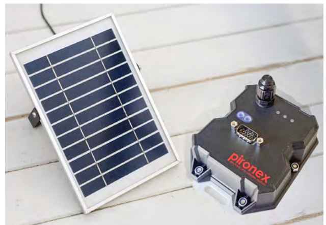
Figure 2: Sensors are supplied with power via the gateway. If a larger number of sensors is required, additional power supply module with a larger solar panel is provided (Source: Pironex)
