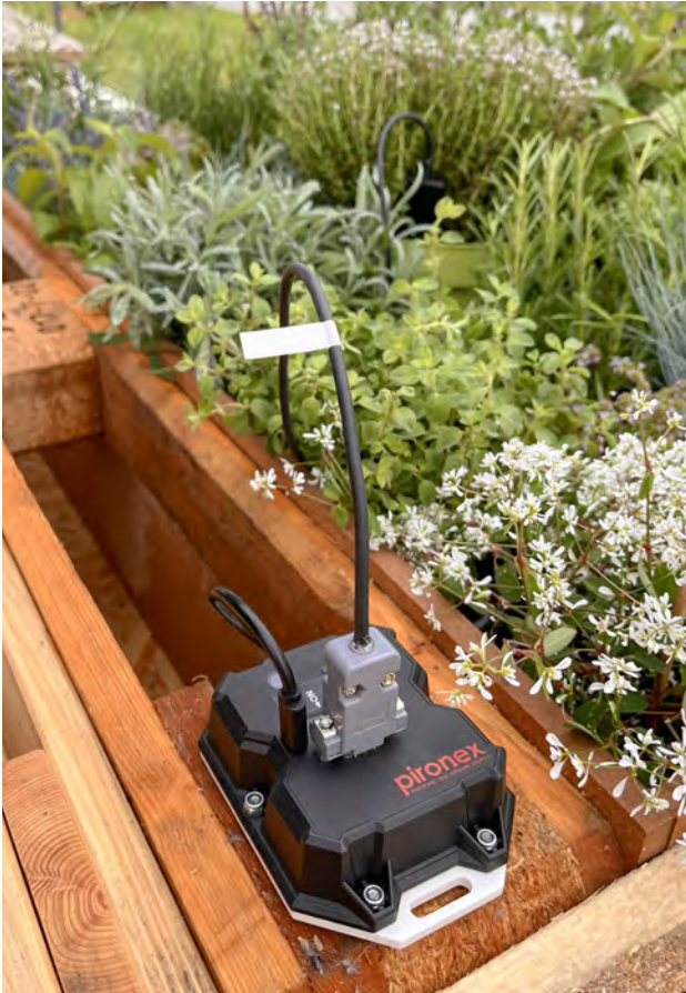
Figure 3: The gateway transmits collected data to the Pironex IoT portal (Source: Pironex)
