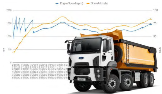
Figure 1: For fleet management, the raw J1939 data can be recorded and decoded using the available J1939 DBC file (Source: CSS Electronics)
