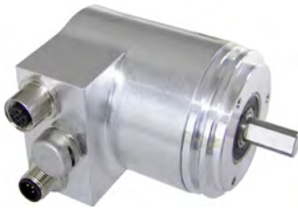
Figure 1: Diverse-redundant encoders have two measurement modules built into a single housing, sharing a common shaft. They do not compare the output from the two measurement channels. Both output signals are transmitted directly to the controller (PLC) to be evaluated there (Source: Posital)
