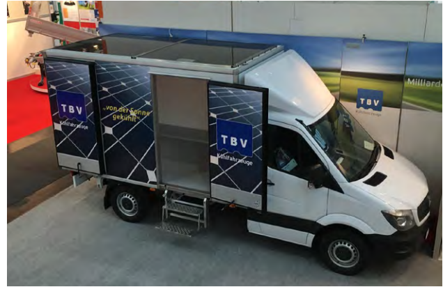
Figure 2: The refrigerated van from TBV uses integrated PV modules to support the refrigeration of the compartment (Source: TBV Kühlfahrzeuge)
