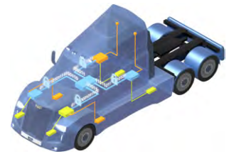
Figure 1: Securing CAN networks in commercial vehicles with NXP Secure CAN transceivers (Source: NXP)
