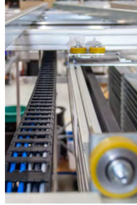
Figure 3: Energy and CAN signals reach the RBG axes through energy chains (Source: Gollmann Kommissioniersysteme)
