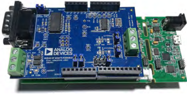
Figure 5: CAN node setup using EVAL-ADM3055E-ARDZ and EVAL-ADICUP3029 (Source: AD)
