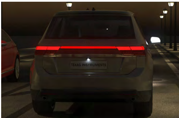
Figure 3: Rear lighting that spans across the length of a vehicle (Source: Texas Instruments)
