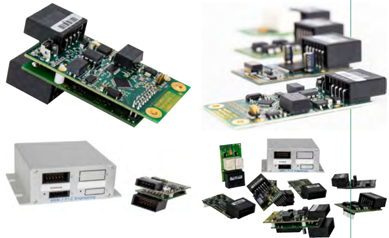
Figure 1: BuildRS comprises two circuit boards; The controller board connects to other devices via CAN and forms the starting point for the unit; the peripheral unit specifies the actual function of the control device (Source: Arrk Engineering)
