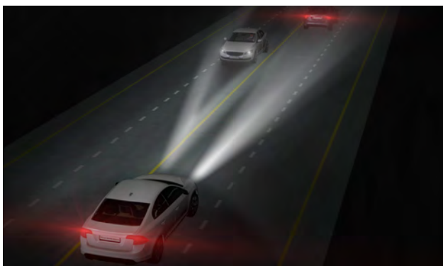
Figure 1: Adaptive headlights adjust the beam shape and illuminate the entire field of view while avoiding glare from oncoming traffic. (Source: Texas Instruments)
