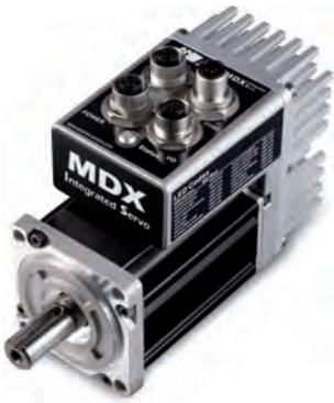
Figure 3: Photo of an MDX integrated servo motor where control electronics are housed at the back of the motor, near the feedback device. No other external electronics package is required to drive or control the motor. The motor includes connectors for power, communications, and I/O. Its on-board controller utilizes the same command interfaces as external motor controllers including CANopen.
