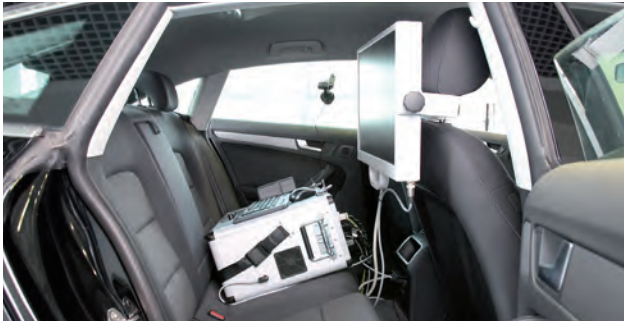
Figure 2: The VTK is put on the back-seats and linked to the CAN-based in-vehicle networks (Photo: Ergoneers)
