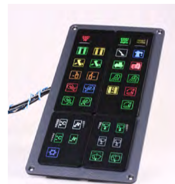
Figure 2: The CAN switching and display units are another mainstay; the photo shows a central control and monitoring panel for a drilling vehicle (Photo: Miunske)
