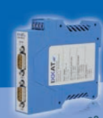
CAN-CR220 CAN repeater (4 kV galv. iso.)
