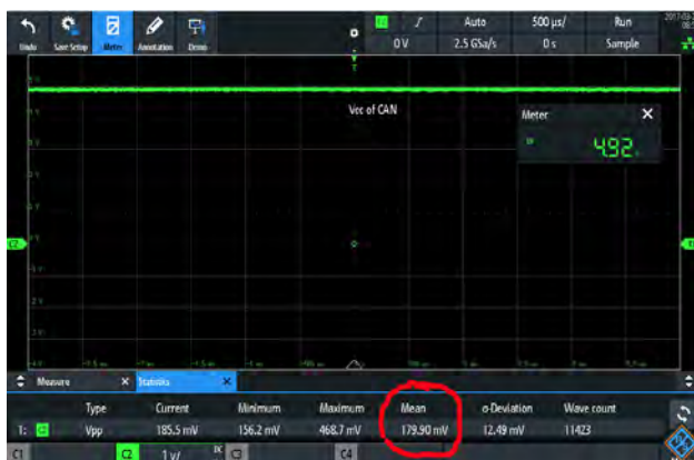
Figure 1: Measurement of DC voltage without any optimized oscilloscope settings (Photo: R&S)
