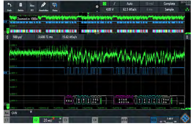
Figure 4: Simultaneous display of analog DC voltage and CAN frame protocol as digital and decoded signal (Photo: R&S)
