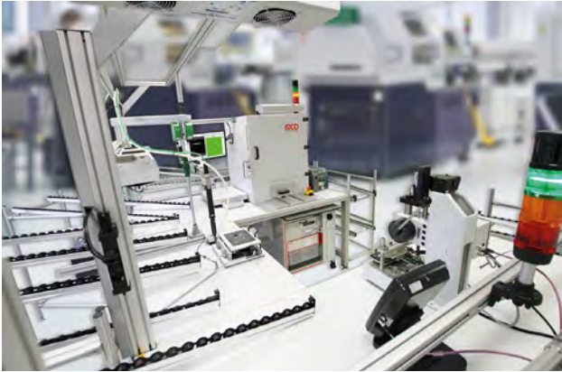
Figure 3: In the foreground (right) the hand-operated press for panel assembly, (centre) the station for final assembly of the control unit, in the background the test cell for optical and electrical testing (Photo: MCD)
