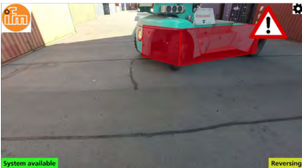
Figure 5: Camera image with a clear warning in the event of objects on a collision course (Photo: Ifm)
