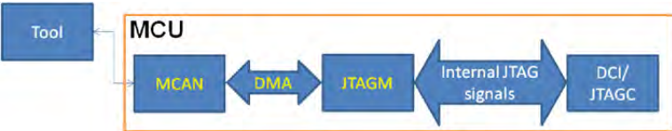
Figure 1: Debug-over-CAN sequence overview (Photo: STM)
