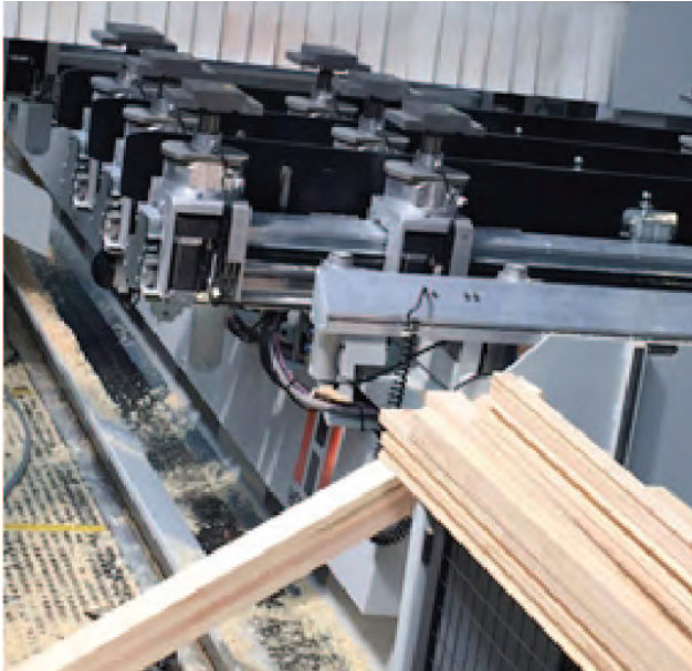
Figure 9: Automatic positioning table for 5-axis CNC machine of wooden window frames (Photo: Servotronix)
