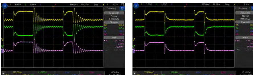
Figure 1: Left: Conventional CAN FD transceiver; right: Denso RSC transceiver (Photos: Denso Automotive Deutschland)
