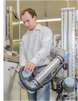
Figure 5: The robot for automated testing processes can be taught by hand-guiding (Photo: Fraunhofer IPA/Rainer Bez)
