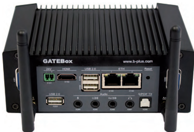
Figure 3: The Gatebox 100 LTE gateway links the in-vehicle networks to the cloud (Photo: B-Plus)
