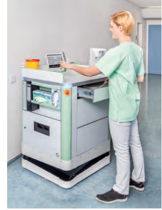
Figure 3: The "intelligent" care cart can be called by care staff and moves autonomously (Photo: Fraunhofer IPA)
