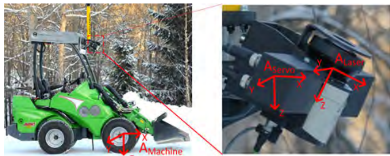
Figure 3: 2D laser scanner (Sick LMS111-10100) installed on an autonomous mobile machine (Photo: TUT)
