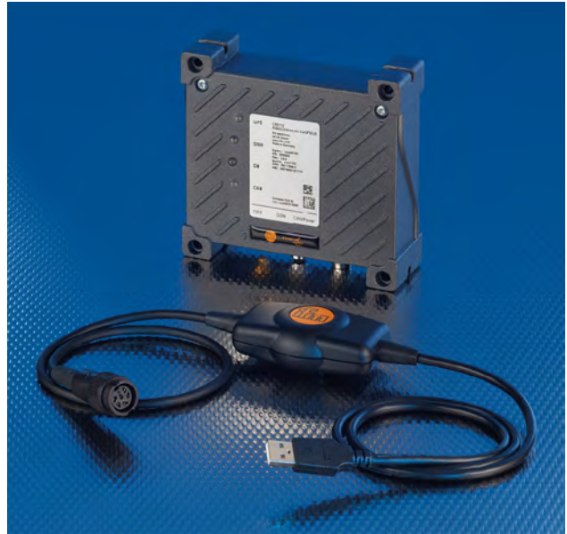
Figure 3: CAN Remote makes it possible to access CAN in a mobile machine via mobile network connection (Photo: ifm)
