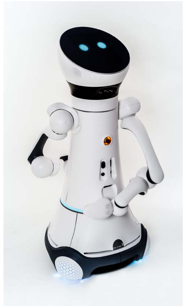
Figure 1: The construction of Care-O-bot 4 allows individual robot platforms to be established for a range of applications (Source: Fraunhofer IPA/Photo: Rainer Bez)
