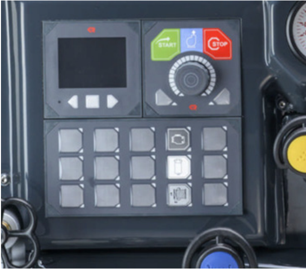
Figure 4: Operation via CAN key panels (Photo: Rosenbauer)
