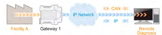
Figure 3: A Virtual PCAN-Gateway in the PC permits the direct access to the CAN traffic in facility A (Photo: Peak)
