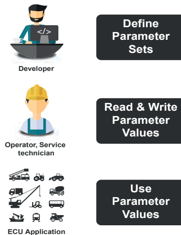
Figure 1: Use-case for parameterization in a mobile machine
