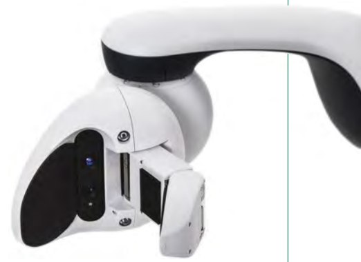
Figure 2: A built-in camera transforms the one-finger hand of the Care-O-bot 4 into a seeing gripper (Photo: Fraunhofer IPA)
