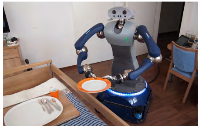
Figure 2: To relieve elderly care personnel from repetitive tasks, Hollie can set the table (Photo: FZI)
