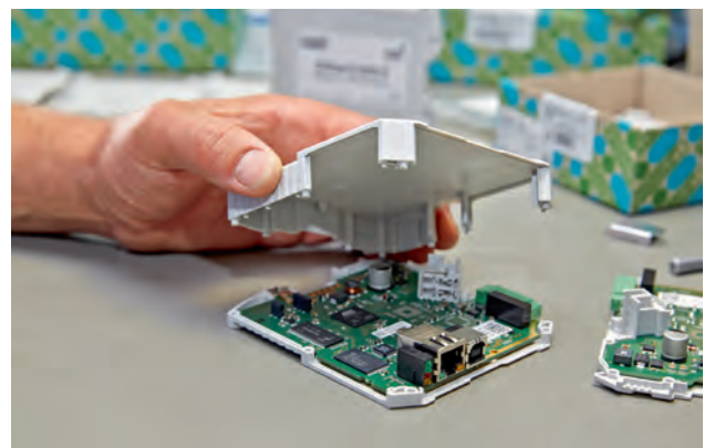
Figure 2: ESD's device manufacturing makes use of the modular electronics housings from Phoenix Contact's ME MAX series (Photo: Phoenix Contact)
