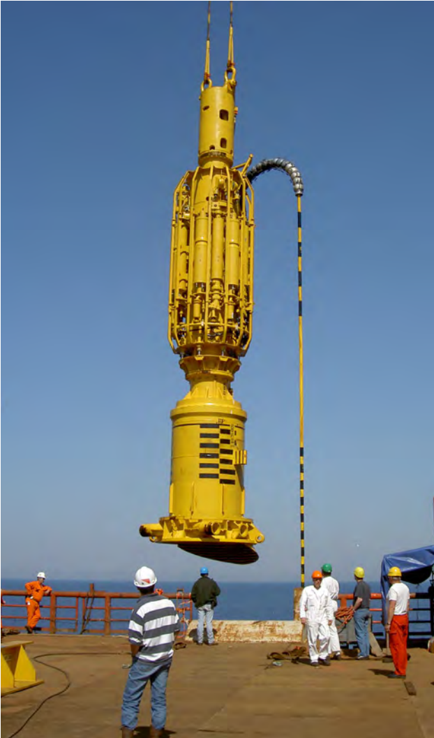
Figure 5: The control and monitoring system of Menck's deep sea hydraulic breaker is mounted directly on the pile hammer; only a single cable for power and communication is needed (Photo: ESD)
