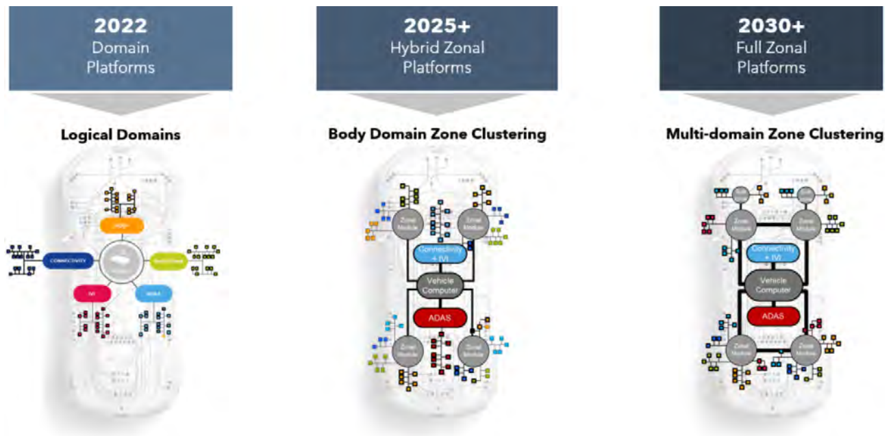
Figure 1: Architectural trend of automotive vehicle networks; from domain-based to zonal-based networks (Source: NXP)
