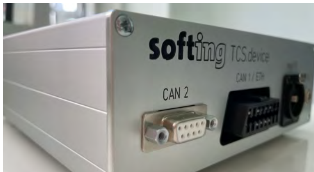
Figure 2: The Softing TCS.device is a configurable diagnostic simulation and can be used as a replacement for real ECUs or vehicles (Source: Softing Automotive)
