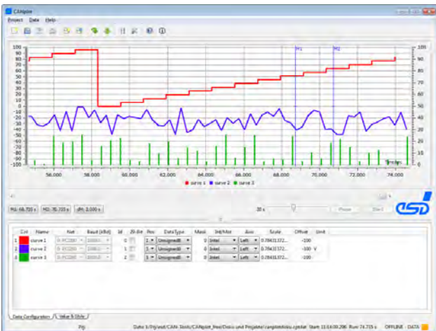
Figure 2: CANplot prepares CAN data and displays them graphically (Source: ESD Electronics)
