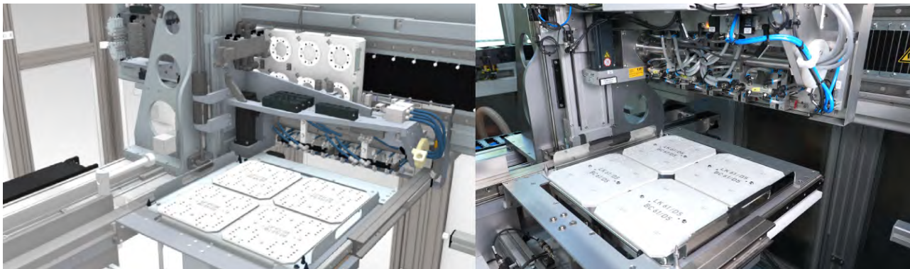
Figure 3: Plastic injection molding machine for pharmaceutical disposables and its digital twin (Source: MI Micro, Otto Männer, Machineering)
