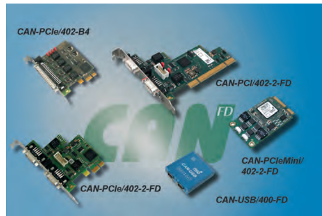
Figure 1: CAN FD boards of 402 series in various form factors (Source: ESD Electronics)
