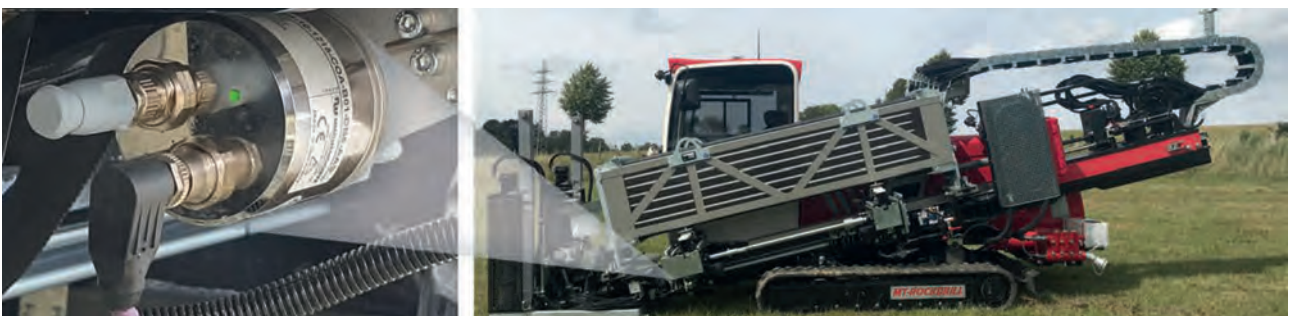
Figure 1: Horizontal drills from AT-Boretec use the WDGA CANopen encoder from Wachendorff for accurate drilling and automated reloading of the drill pipes (Source: Wachendorff)
