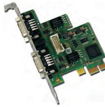
Figure 4: The PC board CAN-PCIe/402-FD according to ISO 11898-1:2015 provides data speed up to 10 Mbit/s and transmits up to 64-bit user data (Source: ESD Electronics)
