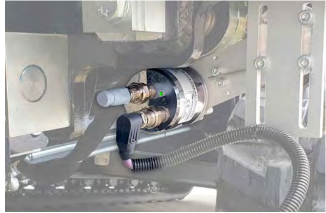
Figure 3: A status LED is integrated in the encoder housing and allows for a rapid diagnosis in the event of an error (Source: Wachendorff)
