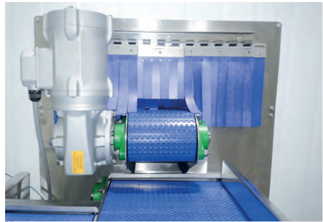
Figure 1 + 2: The NSD Tuph surface treatment provides corrosion protection for drive components in wash-down-optimized cast aluminum housings for the food and beverage industry (Source: Nord Drivesystems)
