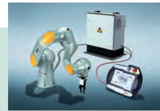
The service robotics modules support the open source ROS software framework and the control module features CANopen functionality (Source: Pilz)
