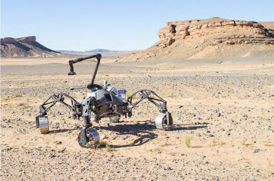
Figure 2: SherpaTT on a rock covered patch of desert in Morocco; an autonomous traverse with a total distance of more than 1 km was successfully conducted in this terrain; path planning, obstacle avoidance and path following are completely calculated on board, without the need for interaction with a ground control station (Source: Jonathan Babel, DFKI)
