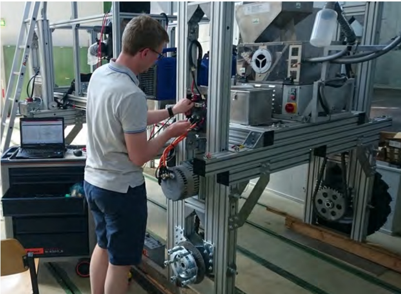
Figure 3: Installation of the drives in the institute workshop (Source: Graf-Syteco)
