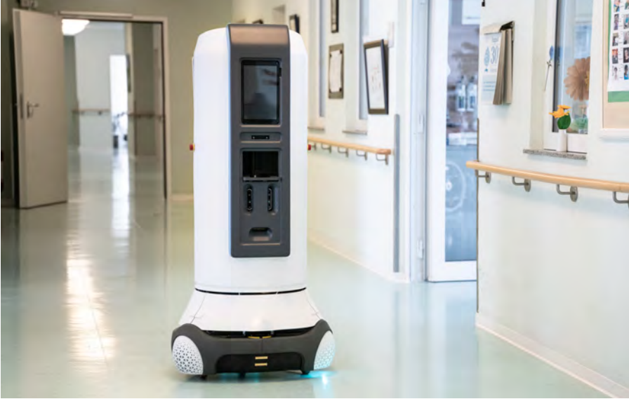
Figure 2: The robotic service assistant is capable of operating in common rooms at care homes and hospitals, where it serves drinks and snacks to the residents or patients (Source: IPA Fraunhofer)
