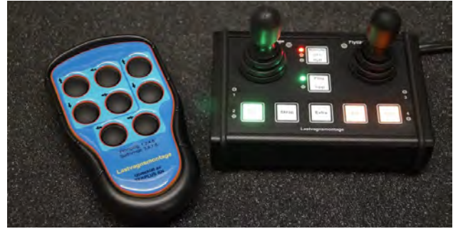
Figure 3: The CAN-based snow plough control on the right and its remote control for external operation on the left (Photo: Klaus Nachtigall, Tekplus)
