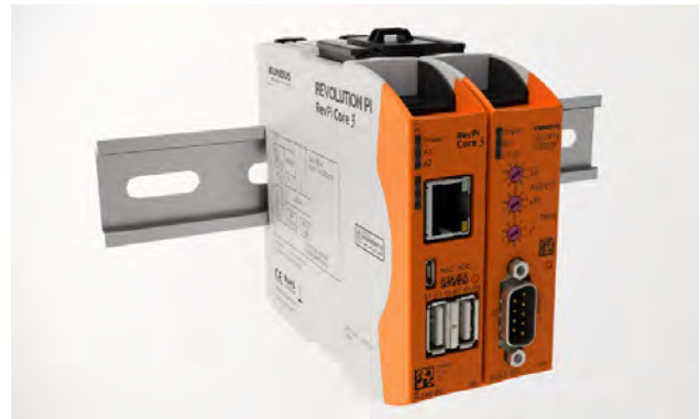
Figure 1: Due to the gateway expansion module for CANopen, The Revpi Core 3 can be integrated into a CANopen network (Photo: Kunbus)
