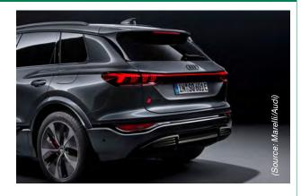
electronic architecture of the system enables refreshing of each image on the OLED panel every 10 ms respectively 100 Hz. This refresh rate is even higher than compared with a usual monitor screen, which refreshes at 60 Hz.
