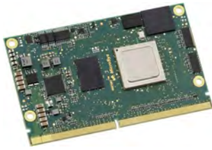
Figure 2: Miriac MPX-S32G274A vehicle network SoM is based on NXP's S32G2 processor (Source: Microsys, Liebherr)
