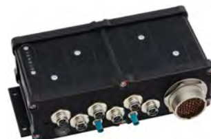
Figure 4: The IP68-rated devices are screwed on to the vehicle frames. They can operate at altitudes up to 5500 m, withstanding temperatures from -40 °C to +70 °C and vibrations up to 6 G (Source: Microsys, Liebherr)
