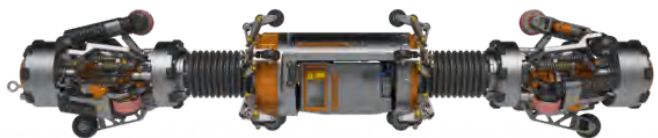
Figure 2: The Agility.mini crawler is dedicated for pipes from 200 mm to 400 mm internal diameter (Source: Optical Metrology Services)
