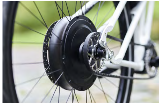
Figure 1: Aximo Pedelec wheel hub motor with a 60-Nm peak torque (Source: Hirschvogel E-Solutions)
