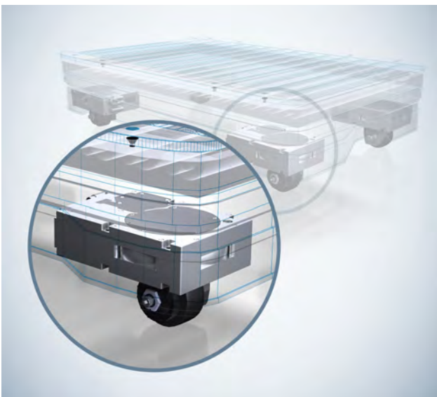
Figure 1: Four Argodrive driving/steering systems, for example, in the heavy version allow a total vehicle weight of up to two tons (Source: EBM-Papst)
