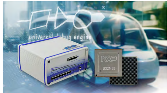
Figure 4: UDE offers an intuitive user interface for debugging and runtime analysis of applications when developing software for the S32N55 (Source: PLS)
