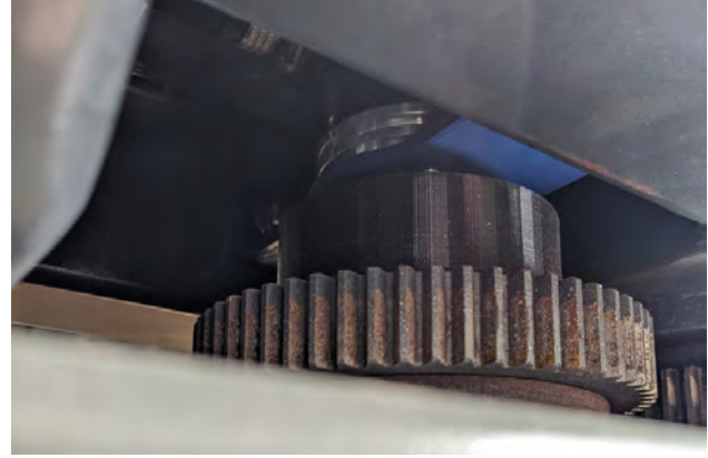
Figure 3 + Figure 4: Important details of the steering: The CANopen WV5800M multiturn rotary encoder records the steering angle so that the vehicle can follow its defined path (Source: Hochschule 21)
