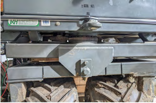
Figure 3 + Figure 4: Important details of the steering: The CANopen WV5800M multiturn rotary encoder records the steering angle so that the vehicle can follow its defined path (Source: Hochschule 21)
