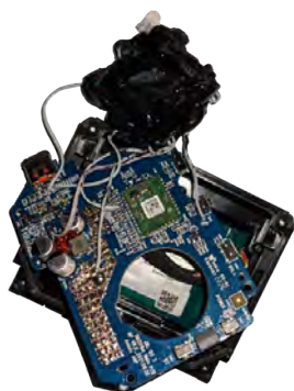
Figure 2: CAN Injector hidden inside a JBL Bluetooth speaker case (the device is powered by the speaker’s battery and hidden in resin) (Source: Ian Tabor)
