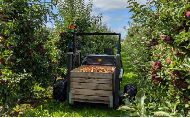
Figure 2: The Aurora harvest assistant will navigate through the rows of trees in an apple orchard and detect and pick up fruit boxes and transport them to a defined unloading point autonomously in future (Source: Hochschule 21)
