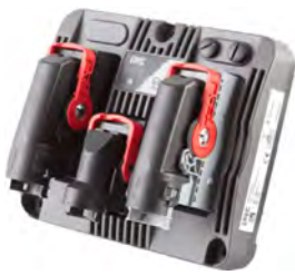
Figure 3: The GL84 is for centralized control system architecture where one commander/central unit controls multiple responders. It has a whopping 27 GND pins for sensors and actuators and CAN1 is also routed to M12 connectors for wiring. (Source: Epec)
