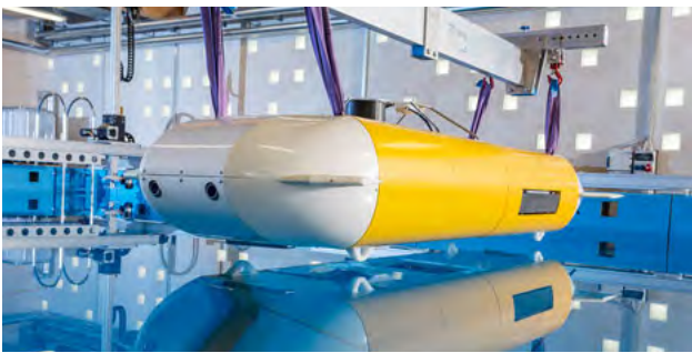
Figure 5: The 3,5-m-long AUV weighs less than 700 kg and provides a slim CAN architecture (Source: Fraunhofer IOSB-AST)
