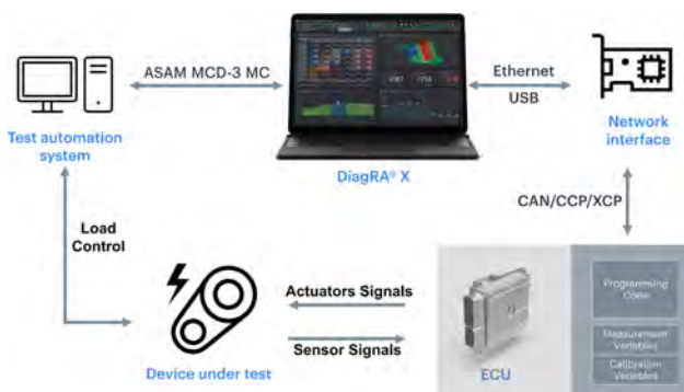
Figure 5: Remote control of Diagra X using ASAM MCD-3 MC (Source: RA Consulting)
