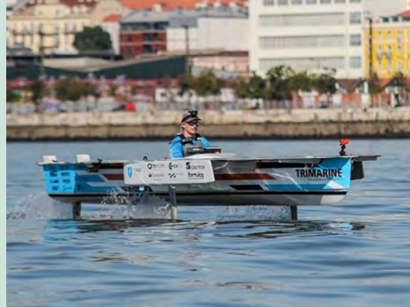
CAN-controlled hydrofoils allow the SR02 boat to get elevated over the water line, thus reducing the drag forces and the energy consumption (Source: Kvaser)
