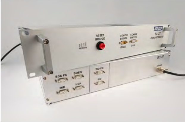
Figure 4 + Figure 5: The TCS-10 CAN switch mounted into a 19-inch rack. These racks are installed in the test basins to accommodate all CAN hardware. (Source: Marin)
