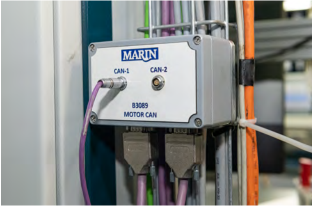
Figure 6: The TCS-10 CAN switch offers the possibility of using a great number of CAN nodes (Source: Marin)
