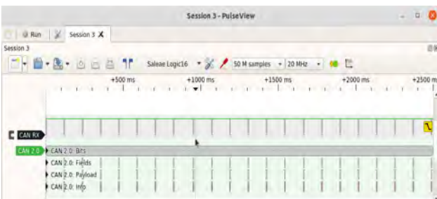
Figure 6: Trace of a pair of CAN frames sent roughly every 100 ms (Source: Ian Tabor)
