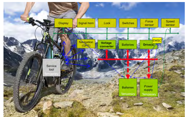
Figure 1: Pedelecs are typically based on CAN and can be modified by the end user (Source: Adobe Stock/CiA)
