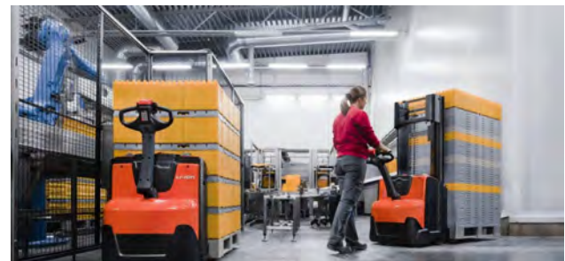
Figure 2: Pedestrian stackers use CAN networks to improve diagnostics and to simplify maintenance; they also reduce the wiring effort (Source: Still)
