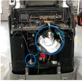
Figure 3: WDGA 58E for detecting the rotation angle of the steering motor (Source: Wachendorff Automation)
