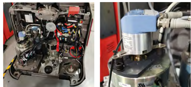
Figure 2: Redundant encoder WDGR 58B for speed detection (Source: Wachendorff Automation)
