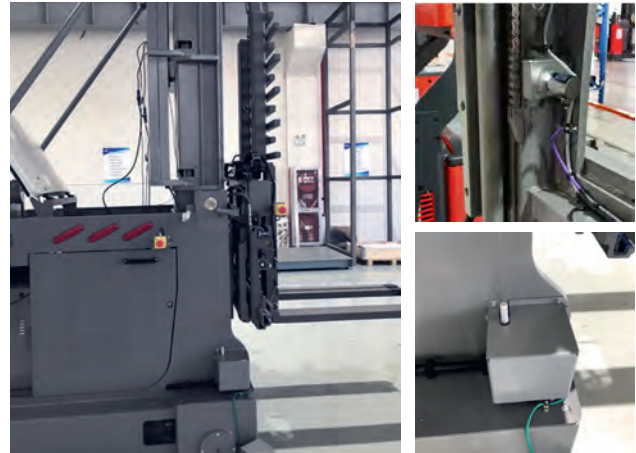
Figure 1: SZG165 draw-wire system and WDGA 36A absolute encoder used for precise positioning of a forklift truck (Source: Wachendorff Automation)
