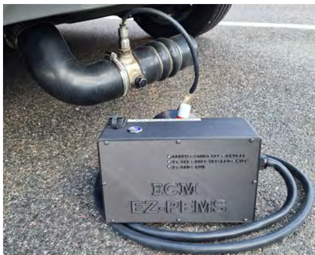
Figure 1: The mobile demonstrator of the miniPEMS compliance tool uses an exhaust adapter to which the sensor fits, without requiring modification of the exhaust (Source: Kvaser)
