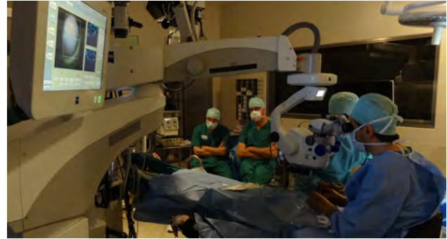
Figure 6: With its surgical microscope with integrated OCT camera, Zeiss gives surgeons better insights into the transparent structures of the eye during surgery. A CAN interface is used in the panel PC. (Source: Zeiss)
