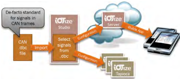
Figure 3: IoTize configuration workflow (Source: Emsa)
