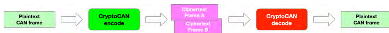
Figure 1: How CryptoCAN encodes and decodes a plaintext CAN frame (Source: Canis Automotive Labs)
