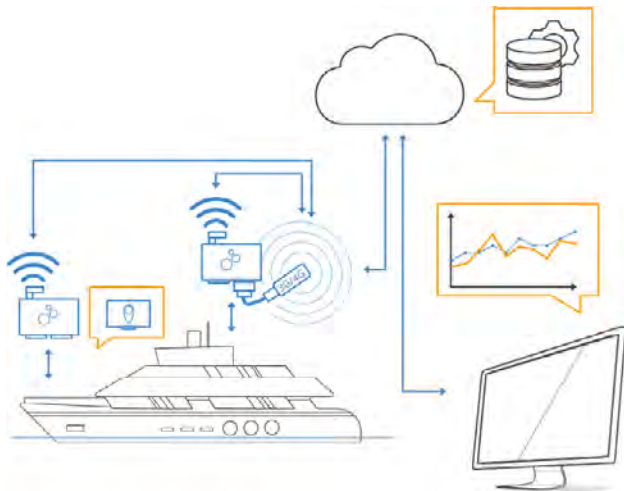
Figure 7: Two CANedge2 units upload MF4 log files from their SD cards via 4G to an AWS S3 server when connectivity is available (Source: CSS Electronics)
