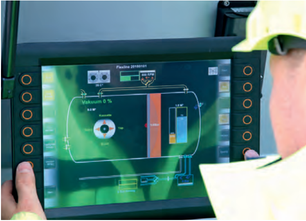
Figure 2: The robust 12-inch display CR1200 installed in the external control cabinet of the vehicle for visualisation and setting of all machine parameters (Source: ifm)
