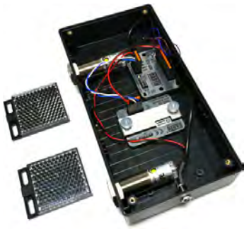
Figure 3: The miniature PLC processes the data and controls the display (Source: RS Components)
