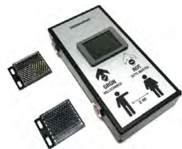
Figure 2: A password-protected CAN touchscreen is used to preset the maximum person limit (Source: RS Components) ▷
