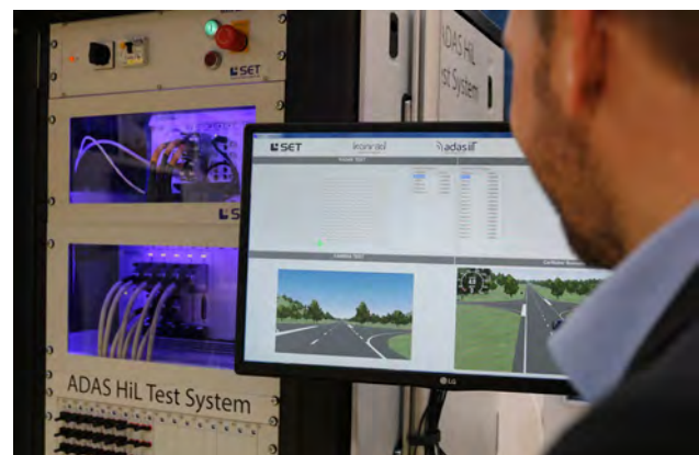
Figure 4: Scenario model IPG on a HIL system (Source: SET)
