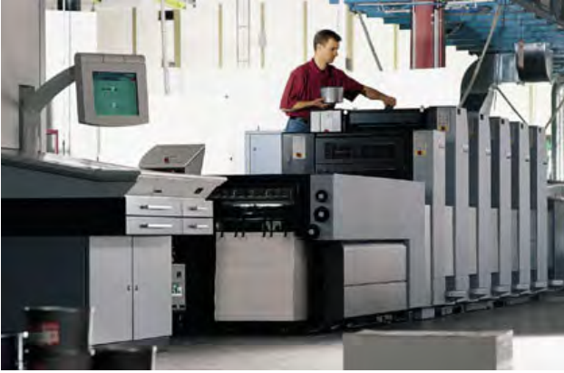
Figure 1: Heidelberg printing machines is one of the early users of CANopen as network to connect add-on devices to its Speedmaster machines (Source: CiA/Heidelberg)
