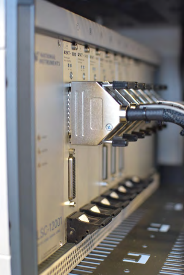
Figure 3: Modular system architecture using SLSC (Source: SET)
