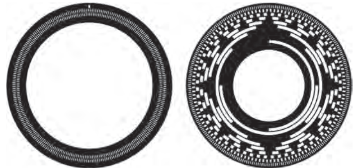
Figure 1: Encoder wheel representations highlight the difference of how positions are indicated between an incremental and an absolute encoder (Source: Schneider Electric)
