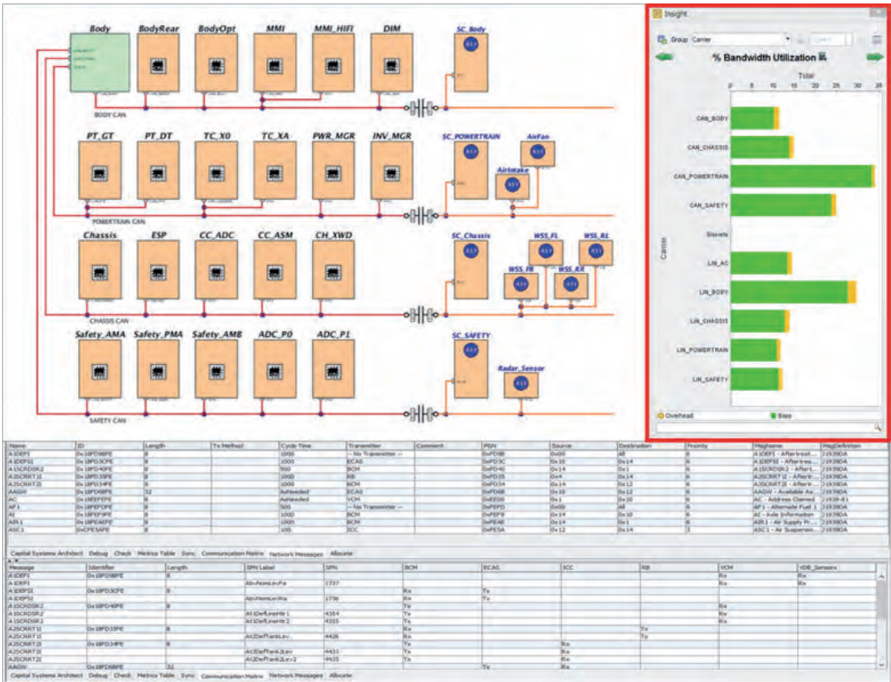
Figure 9: Capital integrates analytics into the design flow so that engineers can evaluate system features such as process loading, network bandwidth utilization, and more (Source: Mentor)
