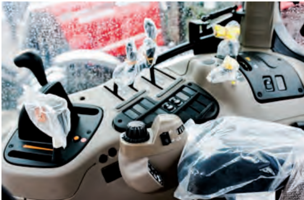
Figure 1: New agricultural tractor cabins are equipped with electronic controls and displays (Source: Mentor)
