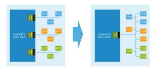
With the introduction of CAN Signal Improvement Capability (CAN SIC), this tradeoff between speed and topology complexity has disappeared (up to a certain degree) and many more nodes can be connected to a single branch. This branch then shares many more vehicle functions which can still be addressed separately through the concept of "virtual branching". When utilizing the option for larger branches it will help the carmaker to reduce cabling complexity, reducing the required number of
