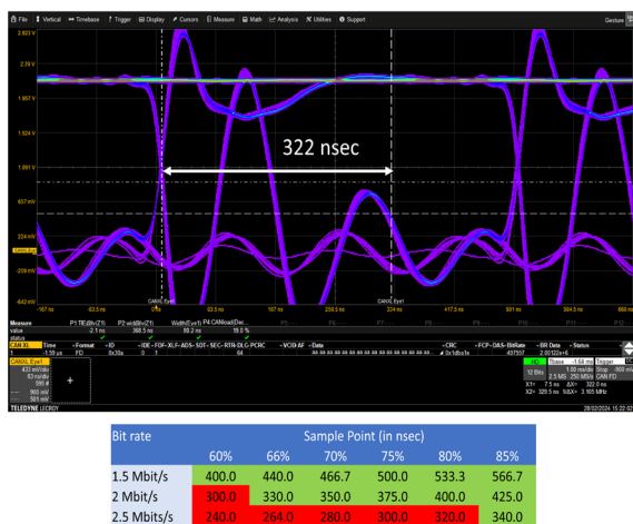
Figure 7: The eye diagram can be used to measure the time until the reflection has leveled off below the CAN signal thresholds.
