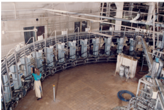
Figure 1: CAN-controlled cow milking and feeding system developed 1992 (Source: STZP / HMS)
