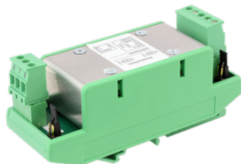
Figure 3: First CAN Repeater presented at the INTERKAMA fair in Dusseldorf in 1992 (Source: STZP / HMS)
