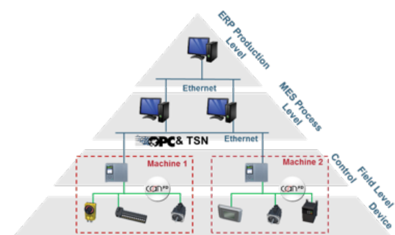
Figure 5: IoT architecture with CAN FD
