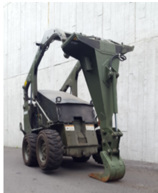
Figure 21: remote controlled skidsteer
