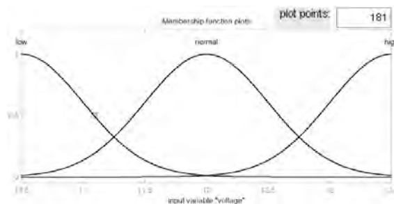
Figure 12: Voltage membership functions has extremum point on 10.5, 12 and 13.5 for low, normal and high level
