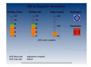
Finally the system shows if the process ended successfully or has been aborted by an error and which kind of error occurred.
