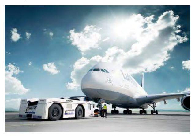
The picture shows the ballasted version of a Challenger 700 with a weight of 70 tons and an Airbus A380 ready to be pushed towards its launch-position.
