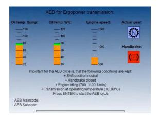
Then the cycle can be started just by pressing the enter-button. This information is transmitted via the CAN bus to one of the PLCs. There it is translated into the SAE J1939 protocol and transmitted to the gearbox-controller.
