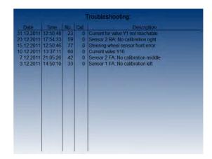
To get a deeper look into the electronic steering system there are separate pages with all the information. From just checking some settings up to calibrating a new angle sensor - everything is possible over the CAN bus.
