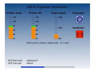
Once the cycle is running its status is displayed to give the operator a direct feedback of the process.
