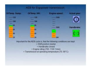
After you are in the AEB-mode the characteristic curve of the gearbox cooling fan is moved to higher temperatures. This is helpful because the transmission's oil has to be heated up to a certain value. The display shows any information the operator needs (temperatures, engine speed, actual gear and the status of the parking brake). It also tells the service engineer what starting conditions are necessary and when they are met.
