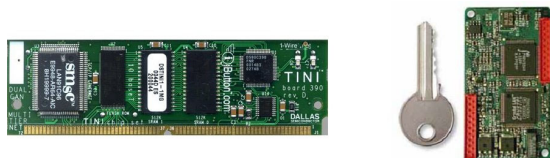
Fig. 10: Examples of embedded web servers, partially available with CAN interface
