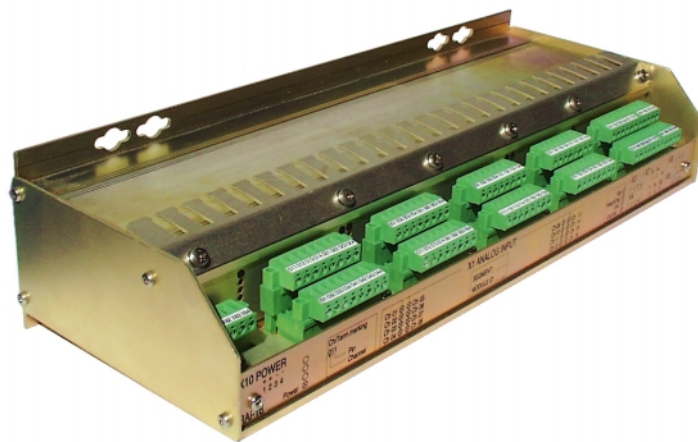
Fig. 3: DPU for 16 channel Analogue Input (Photo: NORCONTROL)
